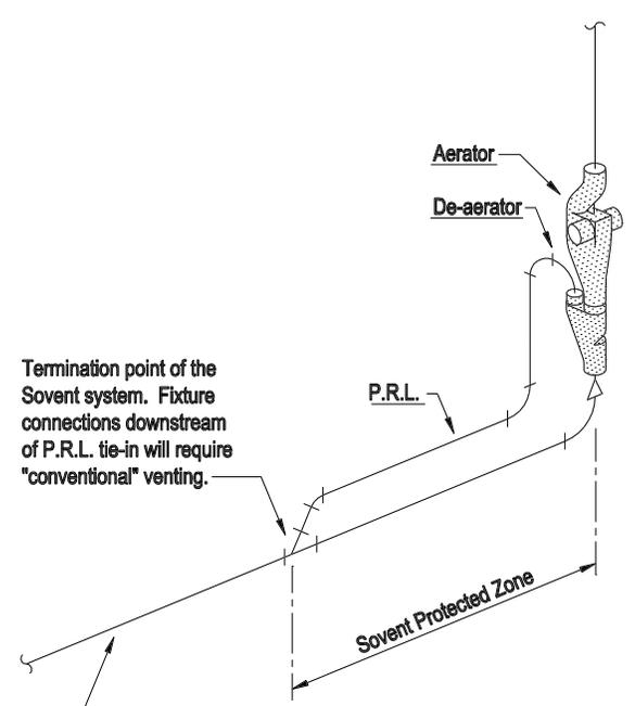
Termination point of the Sovent system. Fixture connections downstream of P.R.L. tie-in will require "conventional" venting.
