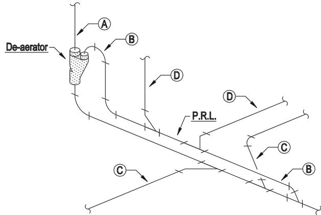
Rough-in height limitations can be reduced by eliminating the Aerator fitting and connecting the lower level fixtures into the horizontal portion of the Sovent system as shown. The De-aerator fitting may be installed above the finish floor providing it remains within 5'-0" of the horizontal drain.
