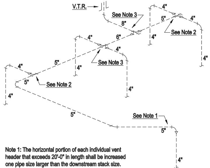
**Note 1:** The horizontal portion of each individual vent header that exceeds 20'-0" in length shall be increased one pipe size larger than the downstream stack size.
