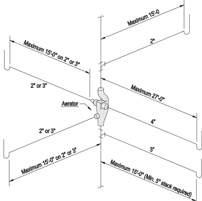
Waste branch developed lengths beyond these limits may require a "conventional" vent or a Pressure Equalizing Line. The vent header or P.E.L. may connect to the Sovent stack a minimum of 3'-0" above the Aerator fitting. P.E.L. Sizing - 4" waste / 2" P.E.L. 3" waste / 1-1/2" P.E.L. - 2" waste / 1-1/4" P.E.L.
