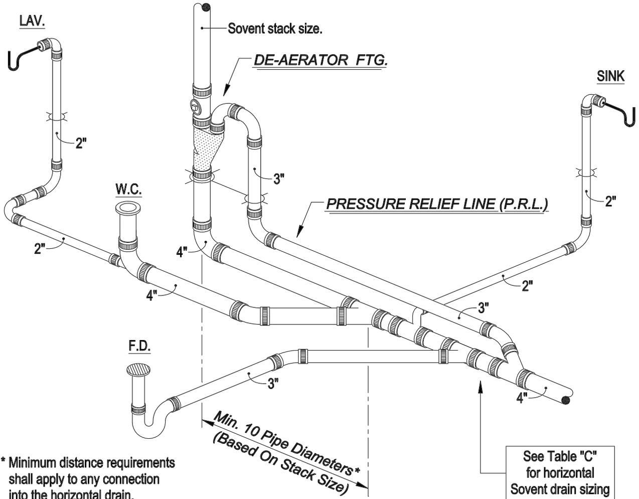
\* Minimum distance requirements shall apply to any connection into the horizontal drain.
