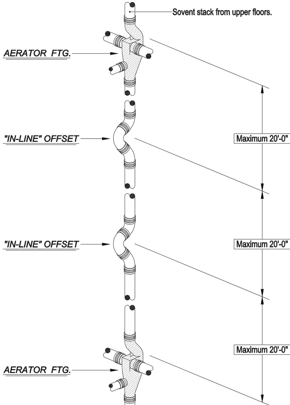
"In-line" Offsets are made by using (1) eighth-bend, (1) quarter-bend & (1) eighth-bend.
