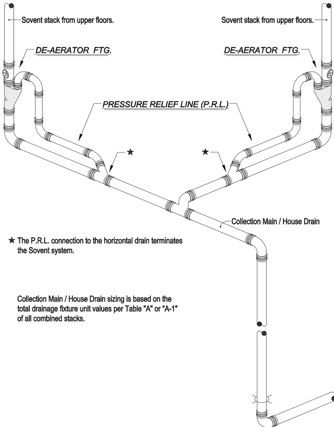
★ The P.R.L. connection to the horizontal drain terminates the Sovent system.
