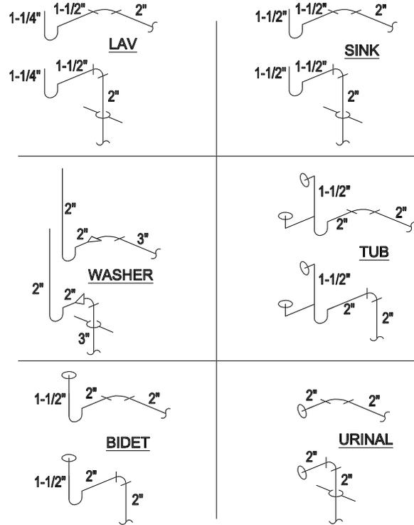
Note: All branch piping located in ceiling or wall areas will be a minimum of 2" in size.
