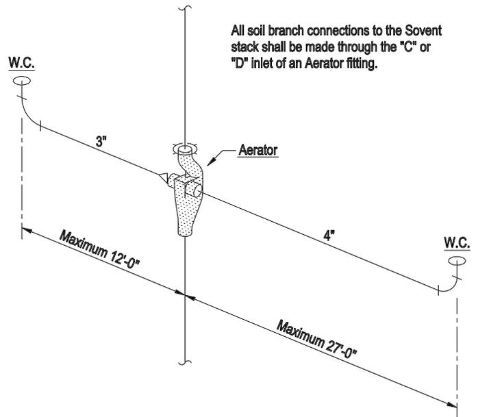
All soil branch connections to the Sovent stack shall be made through the "C" or "D" inlet of an Aerator fitting.
