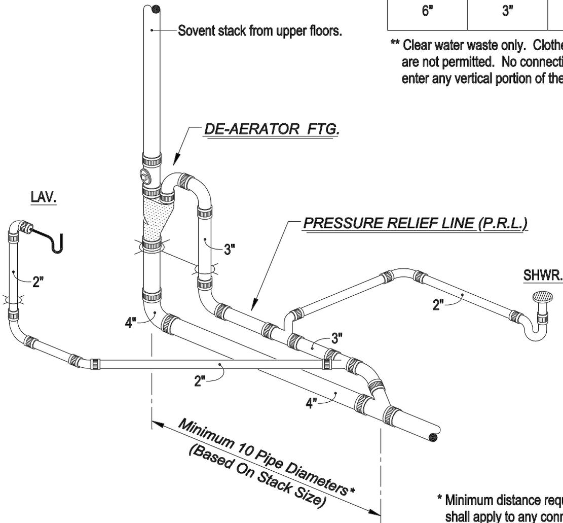
\* Minimum distance requirements shall apply to any connection into the horizontal drain.
