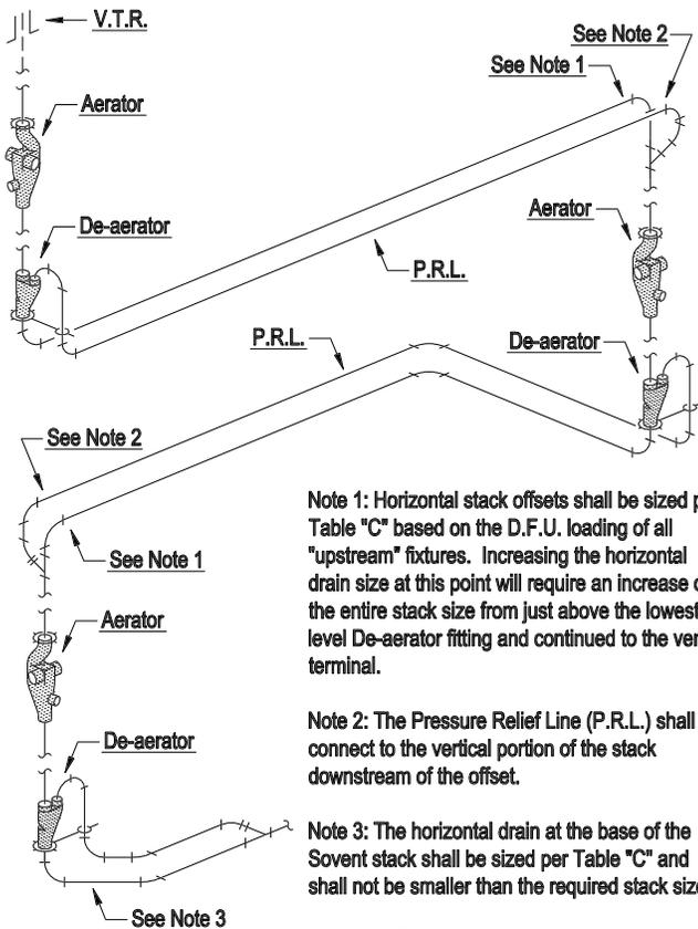
**Note 1:** Horizontal stack offsets shall be sized per Table "C" based on the D.F.U. loading of all "upstream" fixtures. Increasing the horizontal drain size at this point will require an increase of the entire stack size from just above the lowest level De-aerator fitting and continued to the vent terminal.
